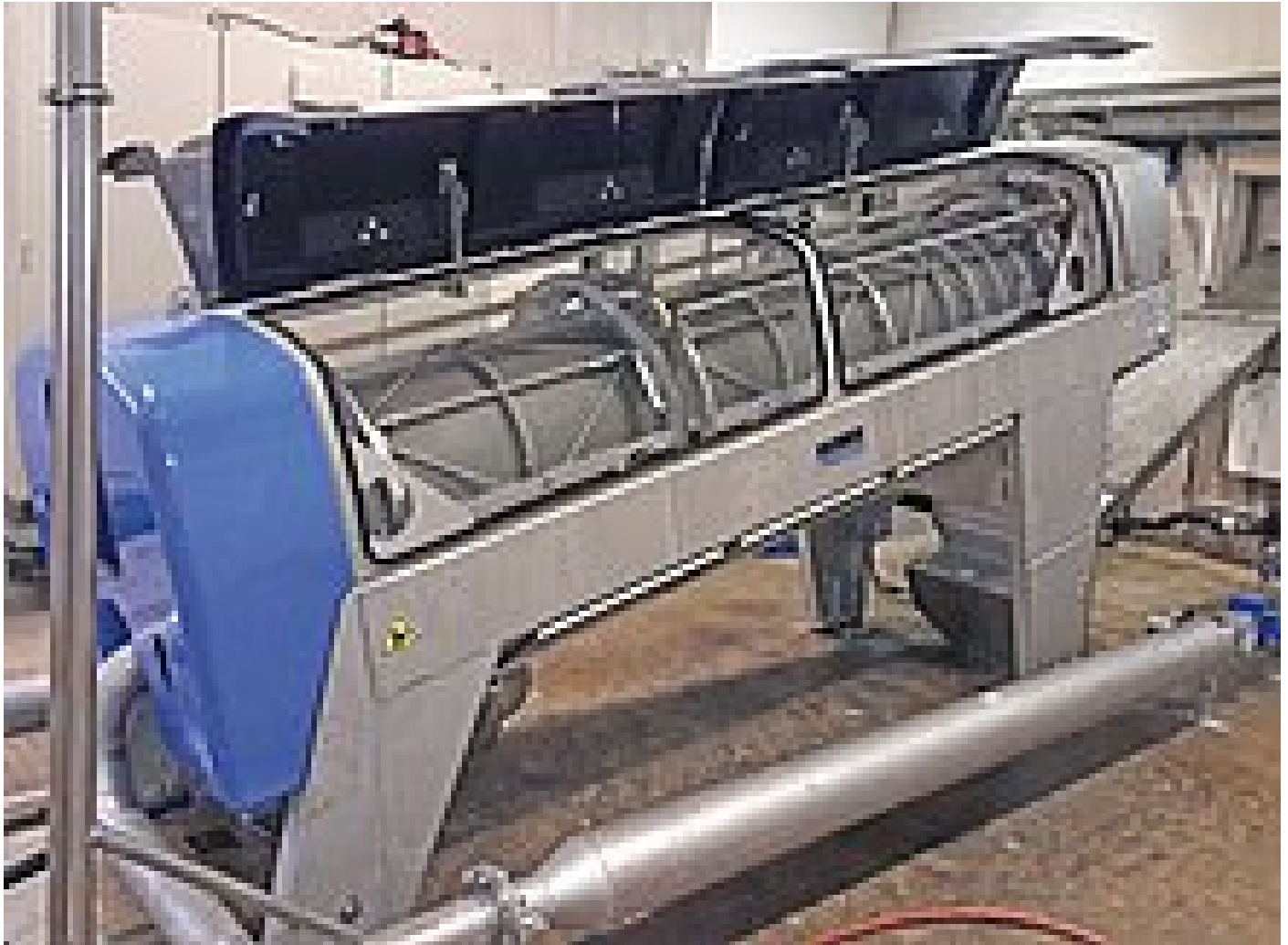
HUBER Screw Press Q-PRESS® 620.2 with open cover
