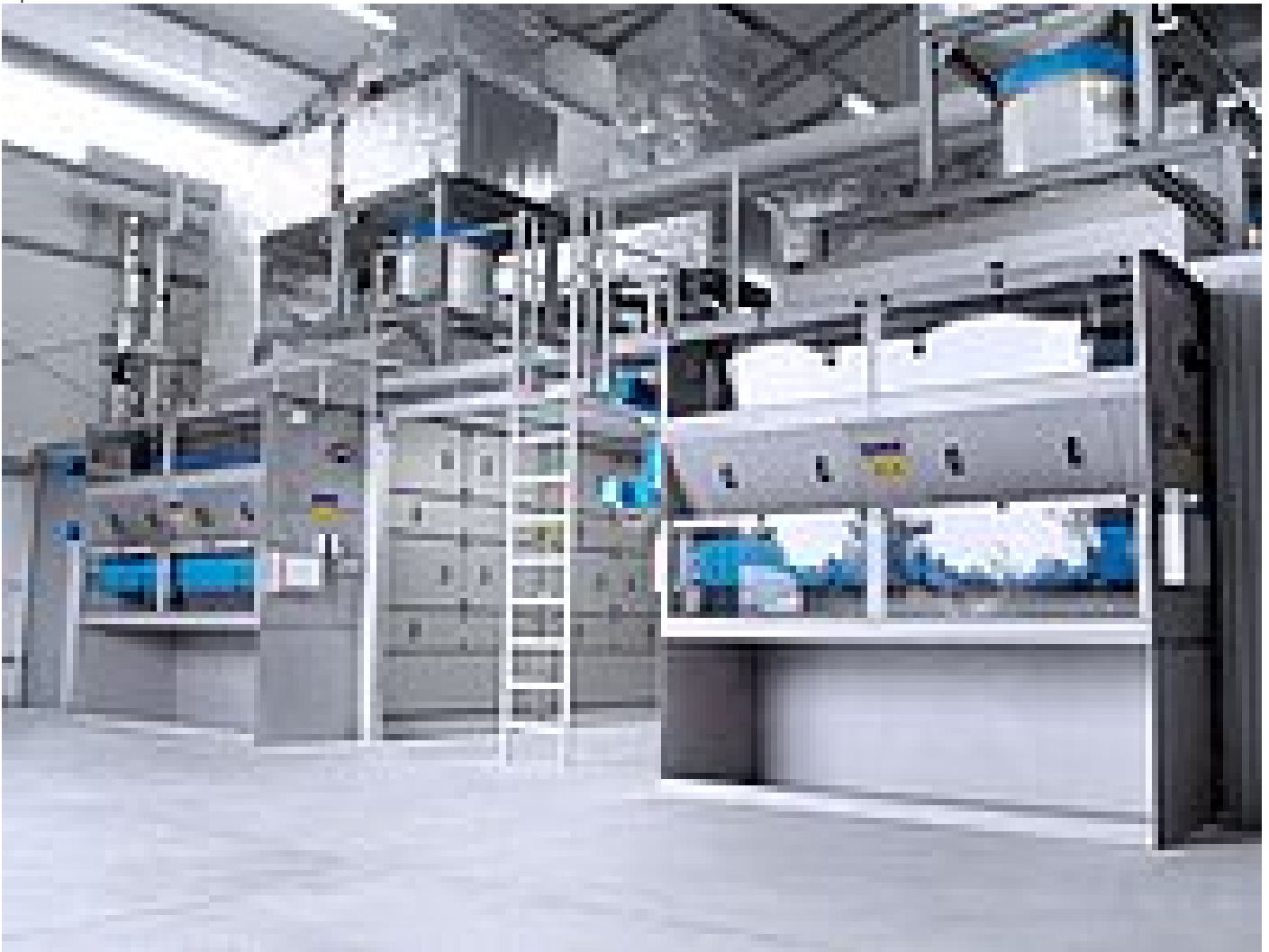
Belt Dryer Installation
