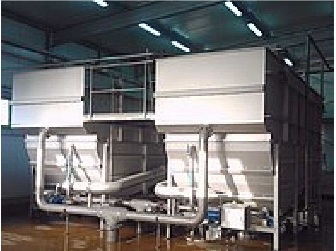
Two sludge flotation plants type HDF S
