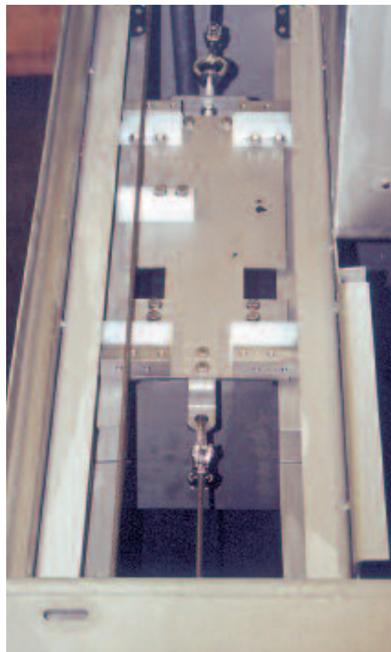
Paddle scraper for grease removal from the grease trap
