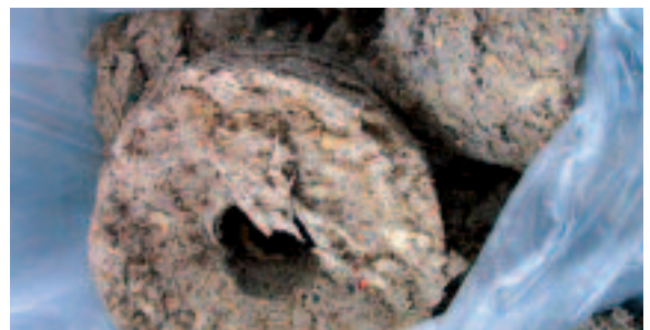
Washed and compacted screenings can be used as fuel for an incinerator
