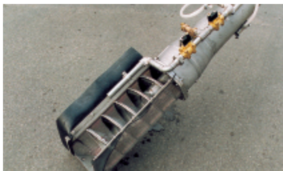
Screen basket of a Ro 9 with integrated screenings washing (IRGA)
